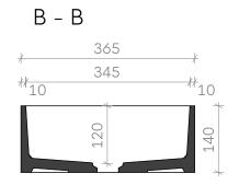
All product sizes are in millimeters and have an informative character. The producer reserves the right to amend the technical specification at any time without previous warning. This sink does not have an overflow hole. Valid from: 22.08.2017
